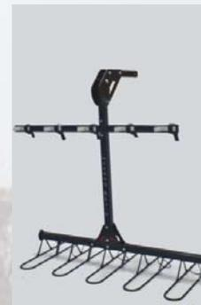
5. To orientate the mid rail looking at the red reflective eyes, while the rack is upside down the short end will be to your right. Attach the mid rail with 2 M10x70 bolts and Nyloc nuts, there are 3 positions to choose from depending on the size of your bikes, a good place to start is to position the mid rail in the centre and adjust if necessary.
