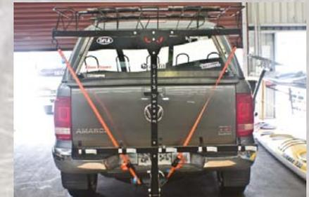
6. (Optional) ratchet straps can be used as 'sway straps', two would be required. Hook one end of the strap to the top rail end plate, and the other to the same side D-shackle point on your hitch, repeat for the other side and tighten to get even tension on each side.
