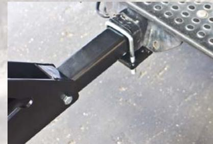
5.a. If your Hitch incorporates an anti-vibration bolt, tighten it and then tighten the lock nut up to your hitch.
