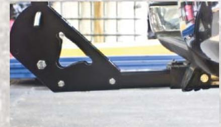
4. When looking at the vehicle insert the anti-vibration bolt from your right side, and tighten firmly, slide the brass spacer over the bolt with the protrusion inserting into the hitch and secure the R clip in the appropriate hole in the anti-vibration bolt.
