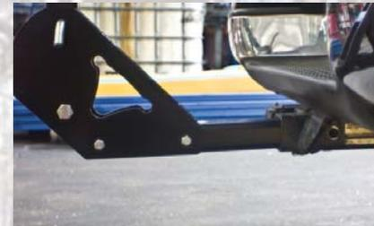
3. Insert the bottom rail into the vehicle's hitch and line up the appropriate hole with the hitch's hole.
