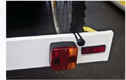
6. (Optional) to attach the Dirty Possum Light Bar, push the bungee ball loop through the orifice and around an appropriate back wheel, securing to the ball on the front of the light board. The light board comes with a 7-pin large round plug, if necessary, use an adaptor or plug straight into your vehicle socket.
