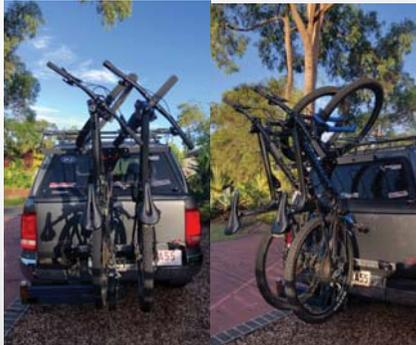
1. Where possible bikes should be evenly distributed from the upright, i.e., for two bikes on a 4-bike rack, the bikes should be in positions two and three, leaving the end positions (one and four) open. Bikes should be loaded Right to Left with the smallest bikes on the outside with the heaviest bikes to the centre.
