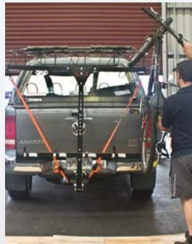
2. To load a bike, facing the rack stand on the right-hand side of the bike, taking the right handle-bar grip with your right hand, and right-hand rear triangle with your left hand lift the front wheel into the basket, pushing the wheel to the front making sure it is resting on the top rail. Lower the back wheel onto the mid rail wheel rest.
