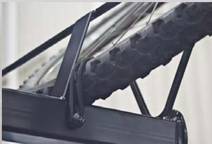
3. Loop the bungee around the front wheel rim and secure to the button at the front. If the Cam Straps are used, wrap the strap around the front wheel rim and pull tight.
