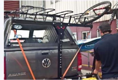
5. Pull the bike down to preload the tyre. While pulling down tighten the cam strap. Repeat for each bike.
