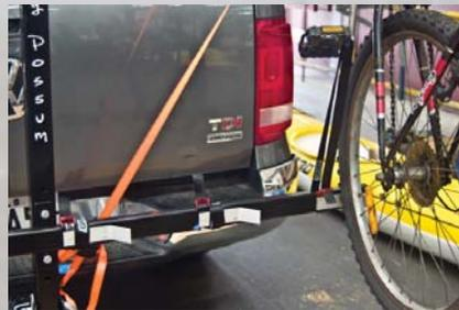
4. Ensure the left-hand side crank arm is pointing downwards, loop the cam strap over the pedal spindle (hard against the crank arm). If necessary, adjust the mid-rail to the centre of the bike wheel.
